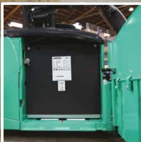
Lateral battery exchange
