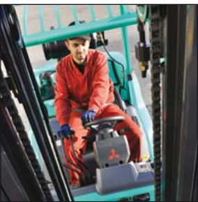
Clear view through mast
