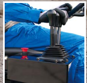
Mechanically isolated ergonomic levers reduce vibration
