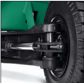
Hydrostatic steering eliminates kickback
