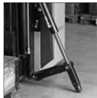
Residual capacity at higher lifts can be increased using side stabilisers (standard on triplex mast).
