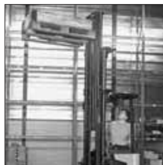
Clear-view mast and diagonal standing position improve visibility and comfort.
