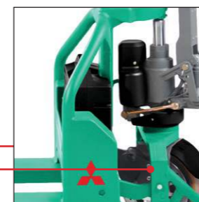
Maintenance-free brushless (AC) wheel hub motor
