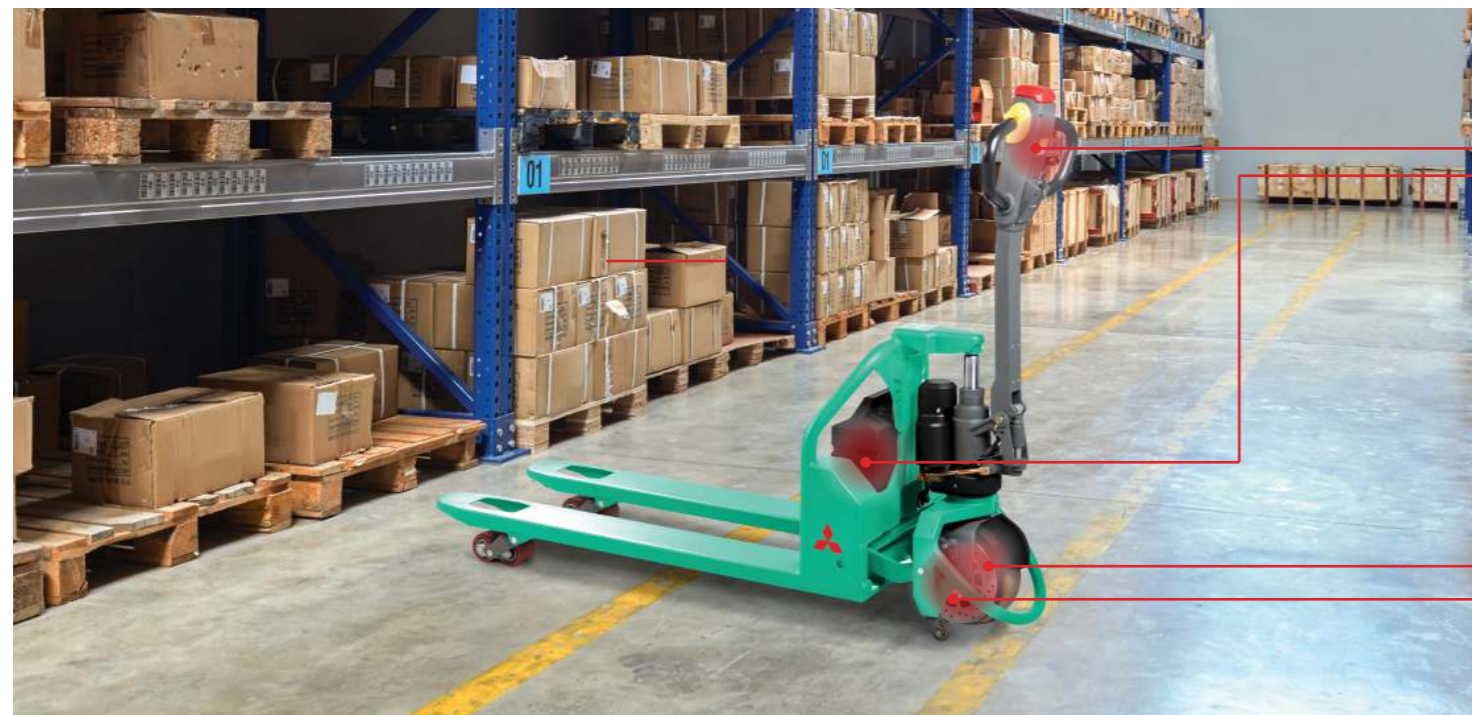
Multi-function ergonomic handle with step-less speed control
