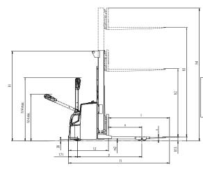
Ast = Working aisle width Ast3 = Working aisle width (b12 <1000 mm) Ast = Wa +  $\sqrt{(16 - x)^2 + (b12 / 2)^2} + a$ Ast3 = Wa + 16 -x +a Wa = Turning radius I6 = Pallet length x = Load wheel axle to fork face b12 = Pallet width a = Safety clearance = 2 x 100 mm
