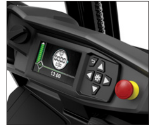
Multifunctional colour display (hourmeter, BDI etc.)
