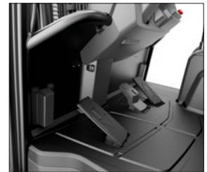
Dual pedal system - forward and reverse. (Option)
