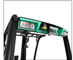
LED working lights, 2 front and 1 rear.
