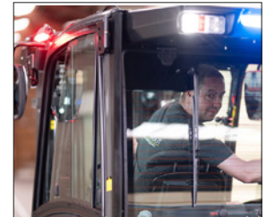
Blue point and red line safety lights
