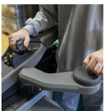
The stand-in power pallet design contains the operator completely within the truck, keeping them protected by the chassis. The stand-in concept also allows for a highly compact footprint. Along with the incredibly tight turning circle, this makes narrower aisle lavouts much more feasible.
