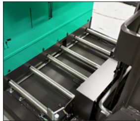
Battery on steel rollers
